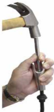
MOUNTING OF TERMINALS IN THE SYNTHETIC ROPE
