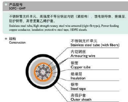
Typical Construction of Submarine Optical Fiber Composite Power Cable
